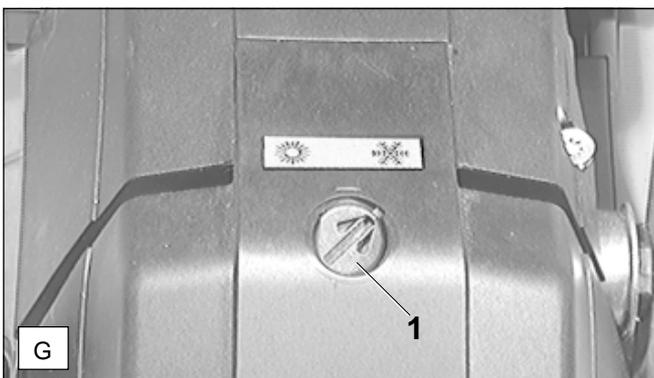
In order to prevent carburetor icing in winter, warm air can be led from the cylinder to the carburetor.
