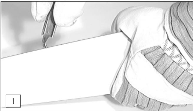
The bearing surfaces of the guide bar must be regularly cleaned and checked for damage.
