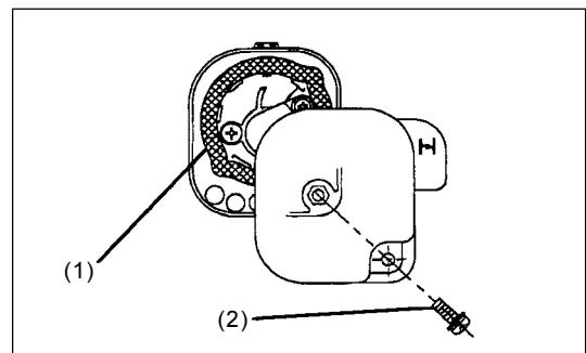
**NOTE:** If there is excessive dust or dirt adhering to the air cleaner, clean it every day. A clogged air cleaner may make it difficult or impossible to start the engine or increase the engine rotational speed.
