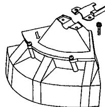
– When using the string head, fit the protector (6) into the protector (1), and tighten them with two nuts (5) and two screws (4).
