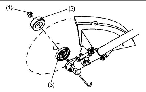
NOTE: The clamp washer (2), and nut (1) are not necessary for mounting the nylon cutting head. The nylon head should go on top of the receiver washer (3).
