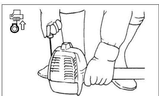
Note: – If the starter knob is pulled repeatedly when the choke button remains at “
