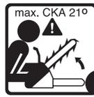
Maximum Computed Kickback Angle (CKA)\* without using the chain brake when using the recommended bar and chain combinations (In this example the CKA is 21°).
