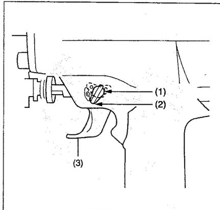
When not operating the tool, always lock the trigger by turning the change lever to the LOCK position.
