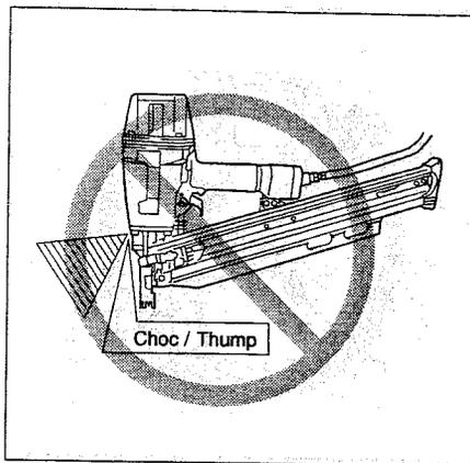
Handle the tool carefully as there is high pressure inside the tool that can be dangerous if a crack is caused by rough handling (dropping or striking). Do not attempt to carve or engrave on the tool.
