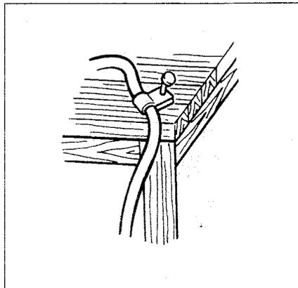
Watch your footing and maintain your balance with the tool. Make sure there is no one below when working in high locations, and secure the air hose to prevent danger if there is sudden jerking or catching.
