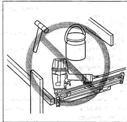
The area should be sufficiently illuminated to assure safe operations. The area should be clear and litter-free. Be especially careful to maintain good footing and balance.
