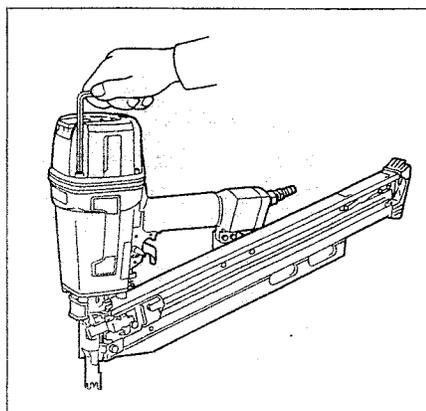
Always check the tool for its overall condition and loose screws before operation. Tighten as required.
