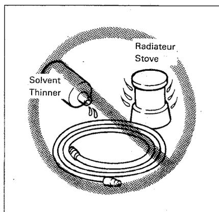
Keep the air hose away from heat (over 60°C, over 140°F), away from chemicals (thinner, strong acids or alkalis). Also, route the hose away from obstacles which it may become dangerously caught on during operation. Hoses must also be directed away from sharp edges and areas which may lead to damage or abrasion to the hose.
