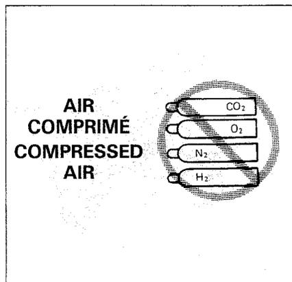
Never use the tool with other than compressed air. If bottled gas (carbon dioxide, oxygen, nitrogen, hydrogen, air, etc.) or combustible gas (hydrogen, propane, acetylene, etc.) is used as a power source for this tool, the tool will explode and cause serious injury.
