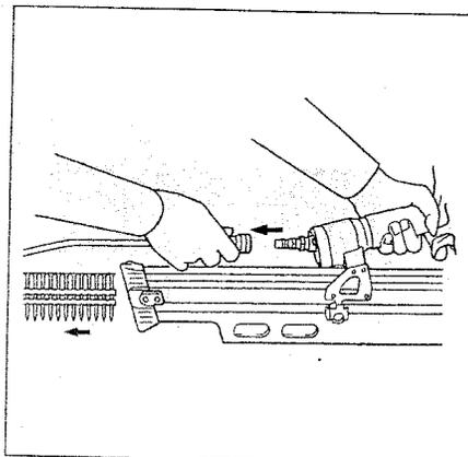
Always disconnect the air hose and remove all of the nails:
