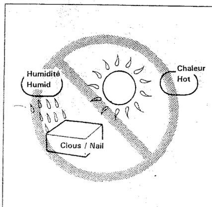
Avoid storing nails in a very humid or hot place or place exposed to direct sunlight.
