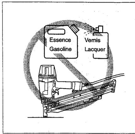
Sparks sometimes fly when the tool is used. Do not use the tool near volatile, flammable materials such as gasoline, thinner, paint, gas, adhesives, etc.; they will ignite and explode, causing serious injury.
