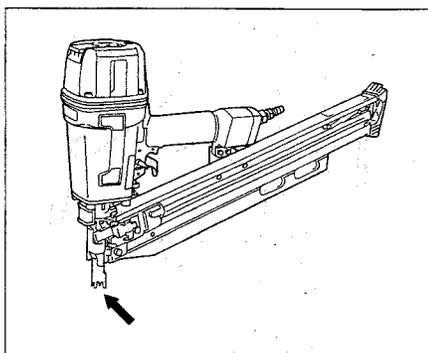
With tool disconnected, make daily inspection to assure free movement of the contact element and trigger. Do not use tool if the contact element or trigger sticks or binds.
