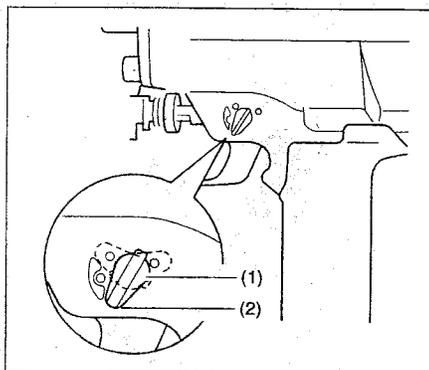
Make sure that the trigger is locked when the change lever is set to the LOCK position.
