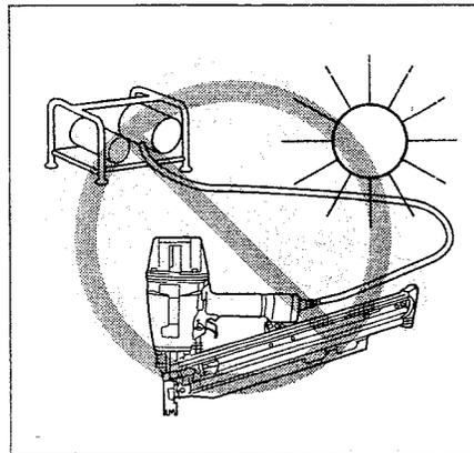
Do not leave the loaded tool or the air compressor under pressure for a long time out in the sun. Be sure that dust, sand, chips and foreign matter will not enter the tool in the place where you leave it setting.
