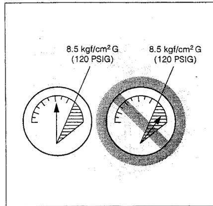
Operate the tool within the specified air pressure of 4.5 — 8.5 kgf/cm<sup>2</sup>G (65 — 120 PSIG) for safety and longer tool life. Do not exceed the recommended max. operating pressure of 8.5 kgf/cm<sup>2</sup>G (120 PSIG). The tool should not be connected to a source whose pressure potentially exceeds 14.0 kgf/cm<sup>2</sup>G (200 PSIG).
