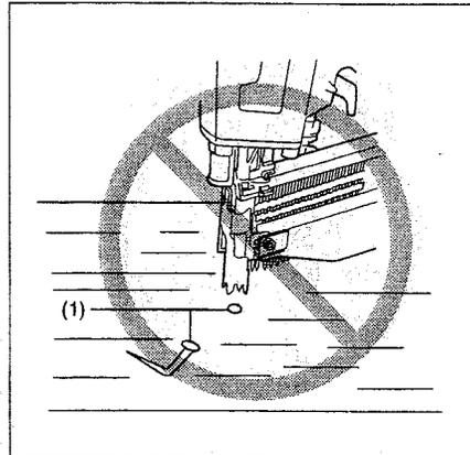
A nail will be bent or the tool can become jammed if you mistakenly nail on top of another nail or strike a knot in the wood. The nail may be thrown and hit someone, or the tool itself can react dangerously. Place the nails with care.
