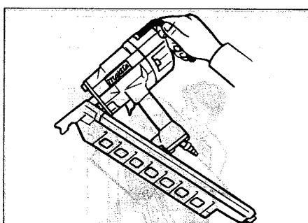
Always check the tool for its overall condition and loose screws before operation. Tighten as required.
