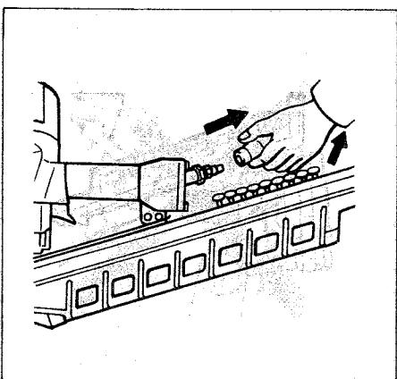
Always disconnect the air hose and remove all of the nails before inspection, maintenance, relocating, or after operation is over.
