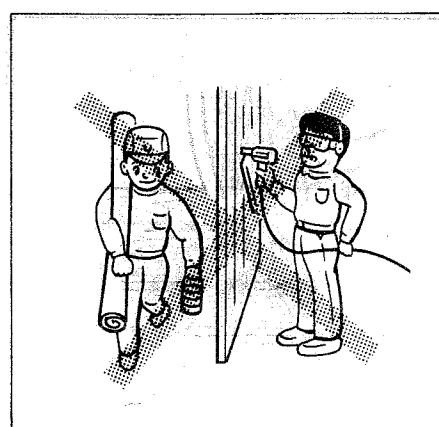
Check walls, ceilings, floors, roofing and the like carefully to avoid possible electrical shock, gas leakage, explosions, etc. caused by striking live wires, conduits or gas pipes.
