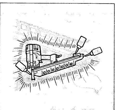
Perform cleaning and maintenance right after finishing the job. Keep the tool in tip-top condition. Lubricate moving parts to prevent rusting and minimize friction related wear. Wipe off all dust from the parts.
