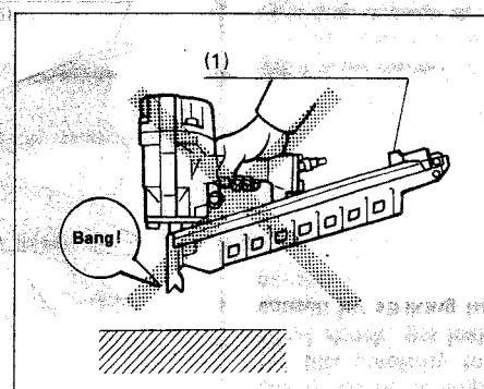
Make sure all safety systems are in working order before operation. The tool must not operate if only the trigger is pulled or if only the contact arm is pressed against the wood. It must work only when both actions are performed. Test for possible faulty operation with nails unloaded and with the pusher locked at fully pulled position.
