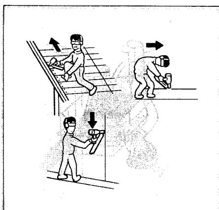
**On rooftops and other high locations, nail as you move forward. It is easy to lose your footing if you nail while inching backward. When nailing against perpendicular surface, nail from the top to the bottom. You can perform nailing operations with less fatigue by doing so.**
