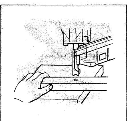
**Hold the workpiece securely. Under nailer impact, the workpiece can fly about dangerously if not held securely in place.**
