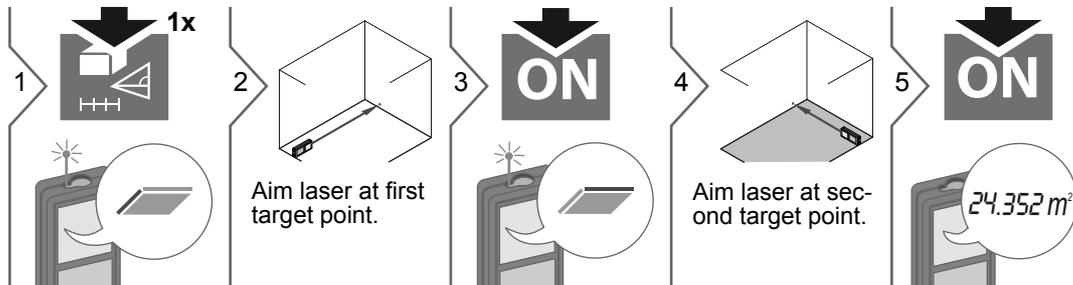
**i** The result is shown in the main line and the measured value above.
