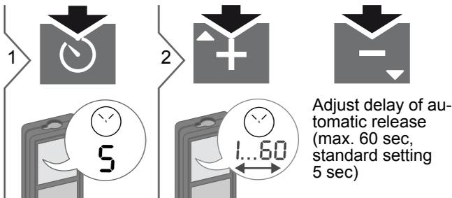
**i** Once the key is released with the laser activated, the remaining seconds until the measurement are displayed in a countdown. The delayed release is recommended for precise aiming e.g. at long distances. It avoids shaking of the device when pressing the measurement key.
