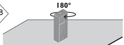
Turn the device horizontally by 180° and place it again on absolutely flat surface.
