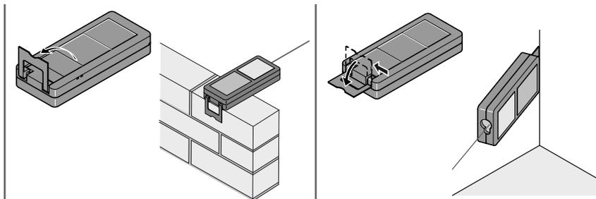
**i** The orientation of the endpiece is automatically detected and the zero point is accordingly adjusted.
