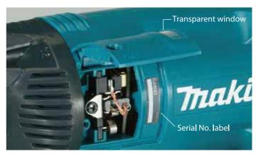
Change from basic spring to Spiral spring without losing the compact body yet extending the working length of Carbon brush.
