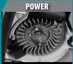
Ignition coil with start-support function stores electrical energy each pull for easier start ups
