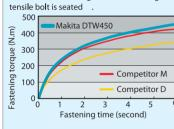
**Test conditions:** M16 High tensile bolt **Fastening torque:** 250N.m
