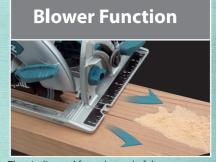
The air directed from the end of the top guide blows sawdust off the cut line ahead.
