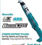
**SPECIFICATIONS Battery Capacities** 14.4V Li-ion Capacity (Driving Shank) Square 3/8" (9.5 mm) No Load Speed 260 RPM 25 - 40 Nm. **Fastening Torque** (221 - 354 in./lbs.) 2-7/8" (73 mm) Width Height (With Battery) 4-1/8" (104 mm) Length (With Battery) 20-1/16" (510 mm) Net Weight 3.3 lbs (1.5 kg)
