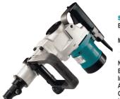
**SPECIFICATIONS** Bit Type: Spline Shank 3/4" Hex, 21/32" Round **Maximum Capacity:** 2" (50 mm) Concrete (TCT) Concrete (Core Bit) 5-7/8" (150 mm) 260 RPM No Load Speed **Blows Per Minute** 2 100 RPM Impact Energy 11.8 J (8.7 ft. lbs) AMPS (120V) 11.0 A **Overall Length** 18-3/4" (476 mm) **Net Weight** 21.8 lbs (9.9 kg)
