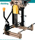
**STANDARD EQUIPMENT INCLUDES:** 5/8" Cutting Chain (A-16570), Chain Bar Assy (133571-3), Wrench 13-17 (781204-0), Oil Supply 100 cc (182229-1)
